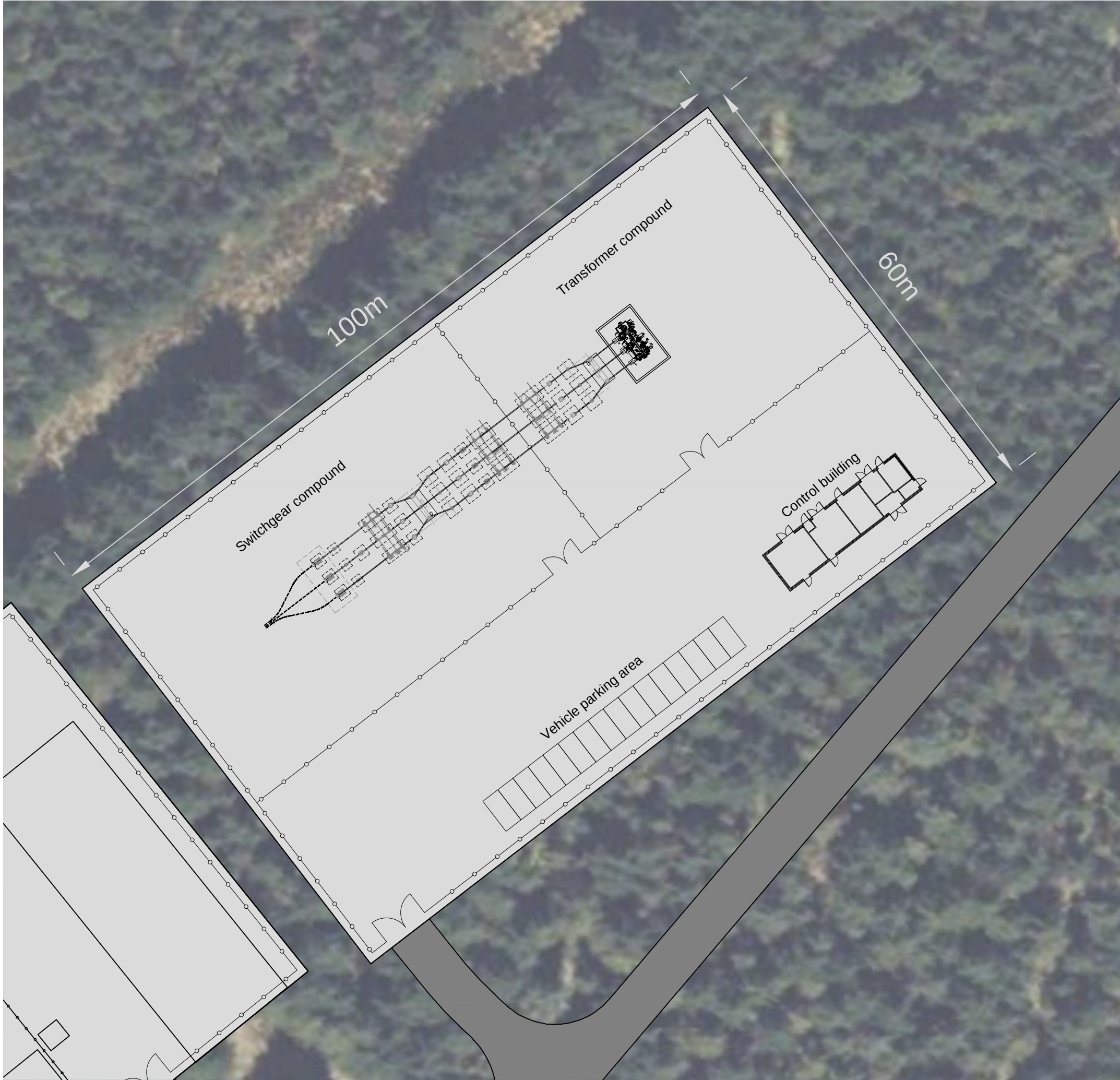
Figure 4.6: Typical Substation Compound Plan
