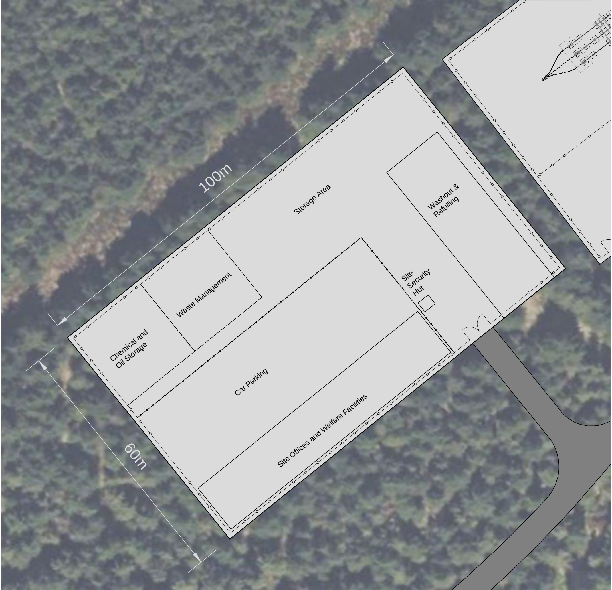
Figure 4.11: Typical Construction Compound Layout Plan
